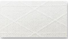
and bond strength to the film. The ZZ Cross-Ply fill of UHMWPE is supported by an Ultra PE ripstop fill yarn for off the charts tear resistance, as well as fill and bias stability. The result is a range of fabrics that will make long lasting cruising sails that hold their shape for years of service to the quality minded cruiser.
